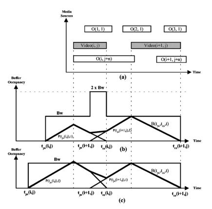
Fig. 5 Relationship between buffer occupancy function, network bandwidth and pre-fetch time for multiple CM objects
