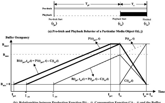
(b): Relationships between Production Function P(t<sub>ps</sub>, t), Consumption Function C(t<sub>cs</sub>, t) and the Buffer Occupancy Function B(t<sub>ps</sub>, t<sub>cs</sub>, t) of a particular Media Object O(i,j)
