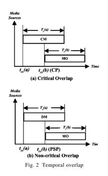
critically overlapped objects in which time instant  $t_{cs(b)}$  is the critical point (CP) of such critical overlap where CM refers to a continuous media object while MO refers to a media object of any type.
